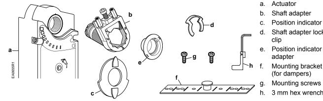
Figure 1. Parts of the ES142 Actuator.
